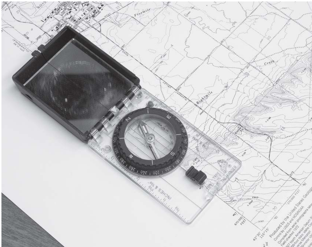
Figure 6-2. Orienting a map with compass.
