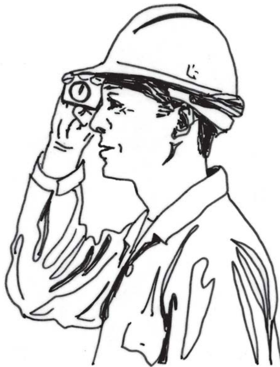
Figure 4-8. Estimating slope with a clinometer.
